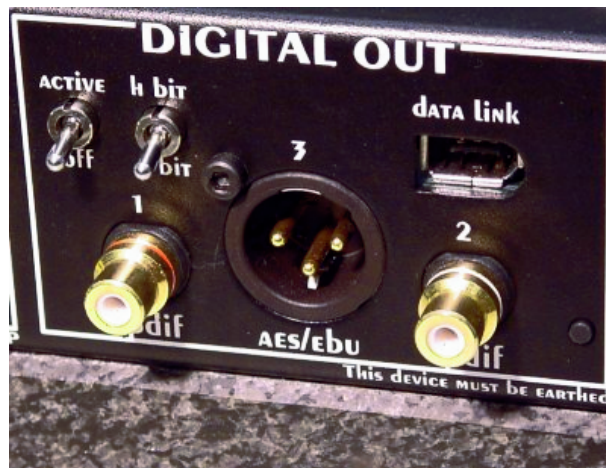
Partial rear view: digital outputs of the VIP
